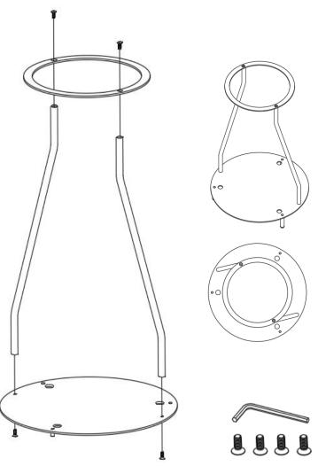
Mount the arms with 2 screws first in the base, do not tighten completely. Align the arms as shown and mount the upper ring with the other 2 screws, do not tighten completely. Center the upper ring from above and when the placement is correct, you can tighten the screws completely, both at the top and bottom.
