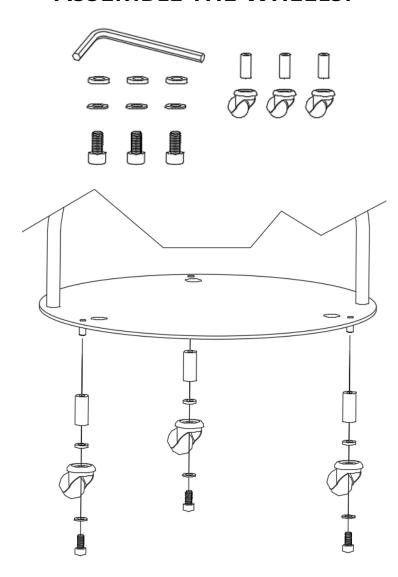
Put on the thin washer, wheel and thick washer on the screw and screw everything onto the short leg. Then screw on the entire wheel set on the underside.
