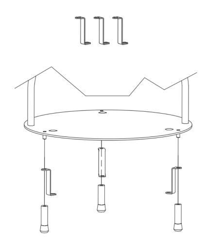
Attach the floor attachment between the leg and the base plate by screwing on the leg. The floor attachment must be directed towards the center. Then fasten the leg frame to the floor with a screw that is suitable for the surface. (Not included)
