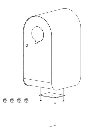
Then mount the bin on the foot plate with 4 nuts and a U-ring 10-key (tools not included)
