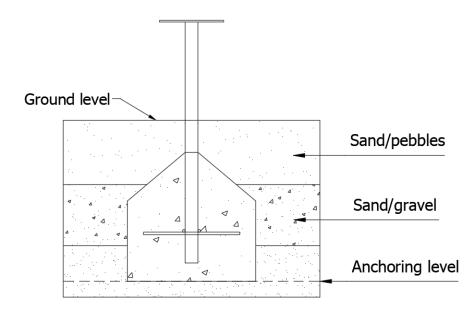
When the foundation has hardened, fill the cavity in the hole with sand / grit to the ground surface, like instruction shows. Place the Popsicle on the mounting plate.
