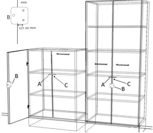
Pair door: Lock stop (A) is mounted (x2 wood screws) under the 3:rd shelf, or under top if the unit only has 3 shelves.
