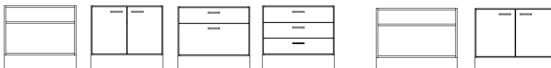
SDÖ80 800x704x570 SDS80 800x704x570 SD80/2L 100% 800x704x570 SD80/3L 100% 800x704x570 SDÖ90 898x704x570 SDS90 898x704x570
