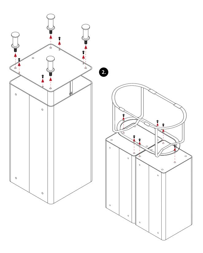
**2.** Turn the frame upside down and unscrew any legs or wheels. Unscrew the mounting screws that attach the bottom plate to the frame.
