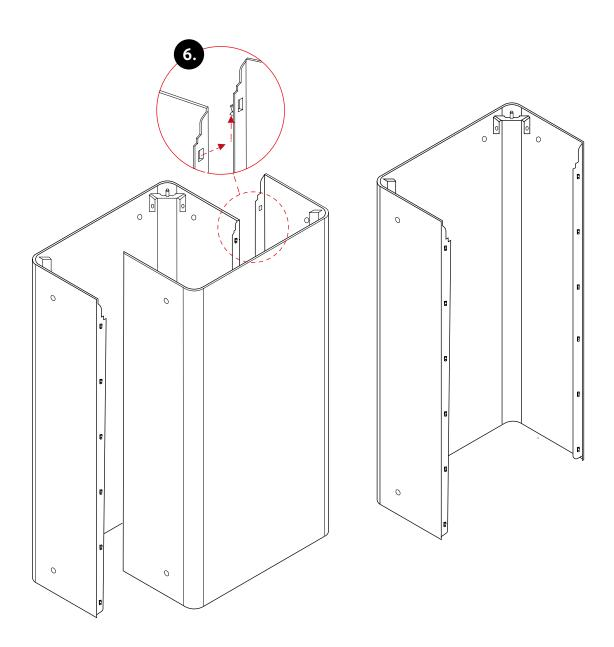
**6.** To split the frame, unhook the hooks by moving one part of the frame upwards. If it gets stuck, try unfolding the upper hook a little. Repeat all the above steps in reverse for assembly.
