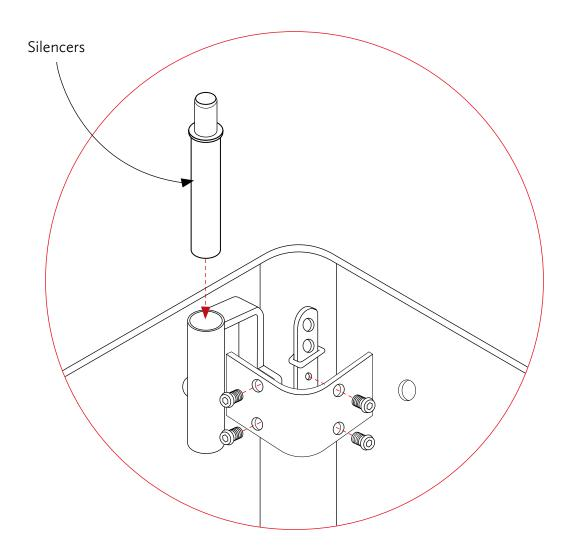
**5.** Remove the silencer. Then unscrew the fastening arm for the bag holder and the damper. Repeat for more.
